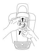
To remove the K-Cup® pod holder from the coffee maker, lift the handle and grasp the top of the K-Cup® pod holder with one hand while pushing up on the bottom of the K-Cup® pod holder from underneath with the other until it releases. After cleaning, align the K-Cup® pod holder with the opening using the two front ribs as a guide and snap into place from the top.
